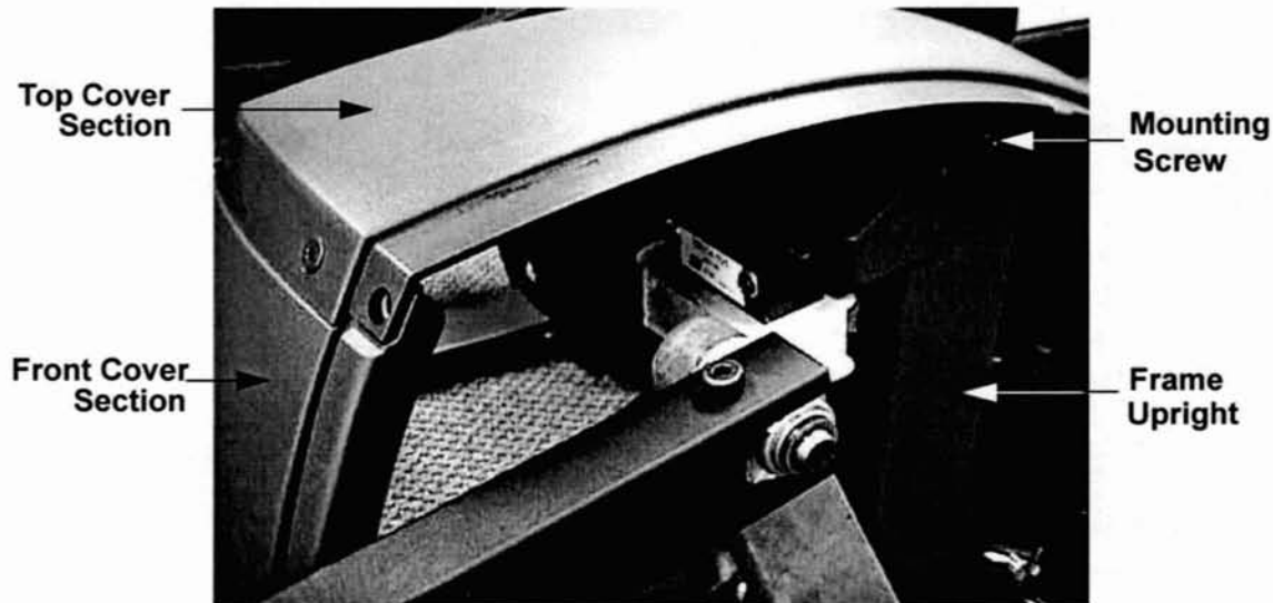
Diagram 7.18 - Top Cover Section (with right & left cover sections removed)
